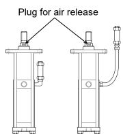
The standard product cannot be used with the rod facing upward.
