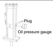
The pressure gauge of a model with pressure gauge is packed separately, and it is shipped. Mount the Power Pack cylinder in the equipment and attach the pressure gauge before oiling. Remove the R1/4 plug next to the "PRESSURE GAUGE" label. Wrap sealing tape around the threads of the pressure gauge and attach it. Oil will not drip if the plug is removed with the pressure gauge port pointing upward, but
