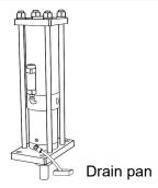
Pipe one-touch fitting to the drain port (Rc1/8) and install a drain pan near the cylinder. It is no pressure. If oil leaks from the piston rod side, it prevents the oil leaking from the rod surface and drains it to the drain port.
