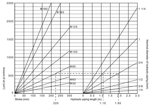
The amount of oil is 1/2 of the capacity calculated from the inner diameter and stroke of the hydraulic cylinder.(In the case of supplying oil to the head side)
