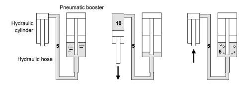
If 10 of oil enters the hydraulic cylinder during fast feed stroke, 5 of oil will return to the pneumatic booster with each operation.
