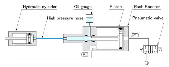
When compressed air is supplied to P1 of the Rush Booster, the piston moves forward and the oil becomes high pressure according to Pascal's principle, and the hydraulic cylinder moves forward with high thrust.
